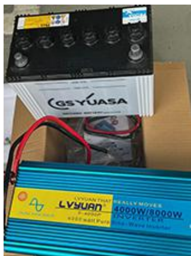
Fig7-5 Converts DC power supply to Ac100 V by connecting to the inverter Starting of Sx Hydrogen sensor by battery
