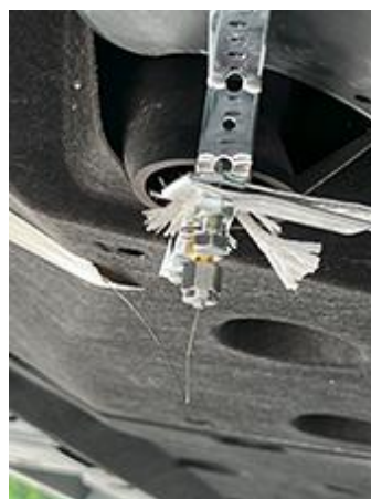
Fig7-7 Adaptor to the exhaust gas sampling from the center of the exhaust pipe of Mirai I
