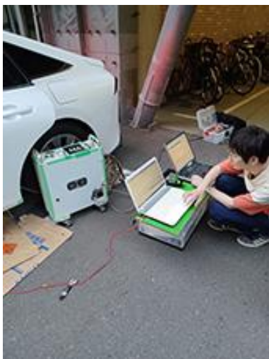
Fig.7-4 H 2 gas monitoring from the exhaust exit of Mirai II
