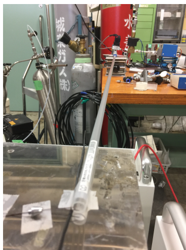
Figure 4. Experimental setup of vertical mixing equipment and sampling gas.
